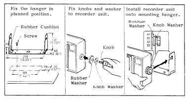
Fig.10 Mounting the Recorder Unit
